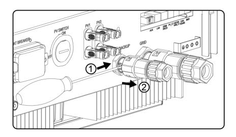
To disassemble the grid connectors from the SMILE5-INV, unscrew the grid connector counterclockwise until it can't be rotated and unplug it.
