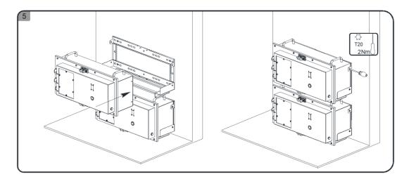
Mount the expansion battery M4856-P downwards as follows.
