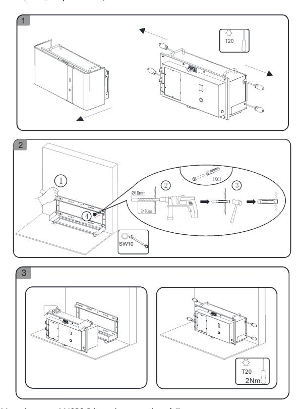
Mounting more M4856-P batteries upwards as follows.
