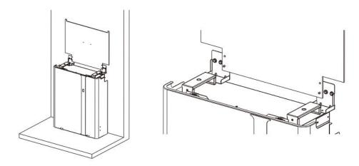
Locate the left position plate to the wall bracket of M4856-P.
