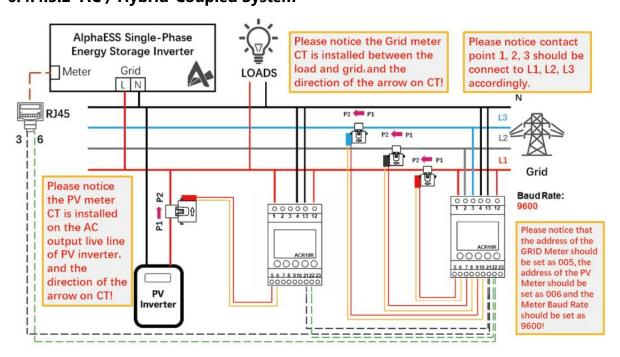
ACR10R three-phase Connection (AC / Hybrid-Coupled System)
