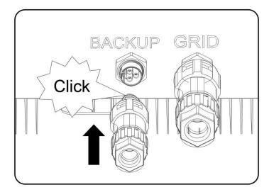
PS: Follow-up steps for disassembling the AC connector:
